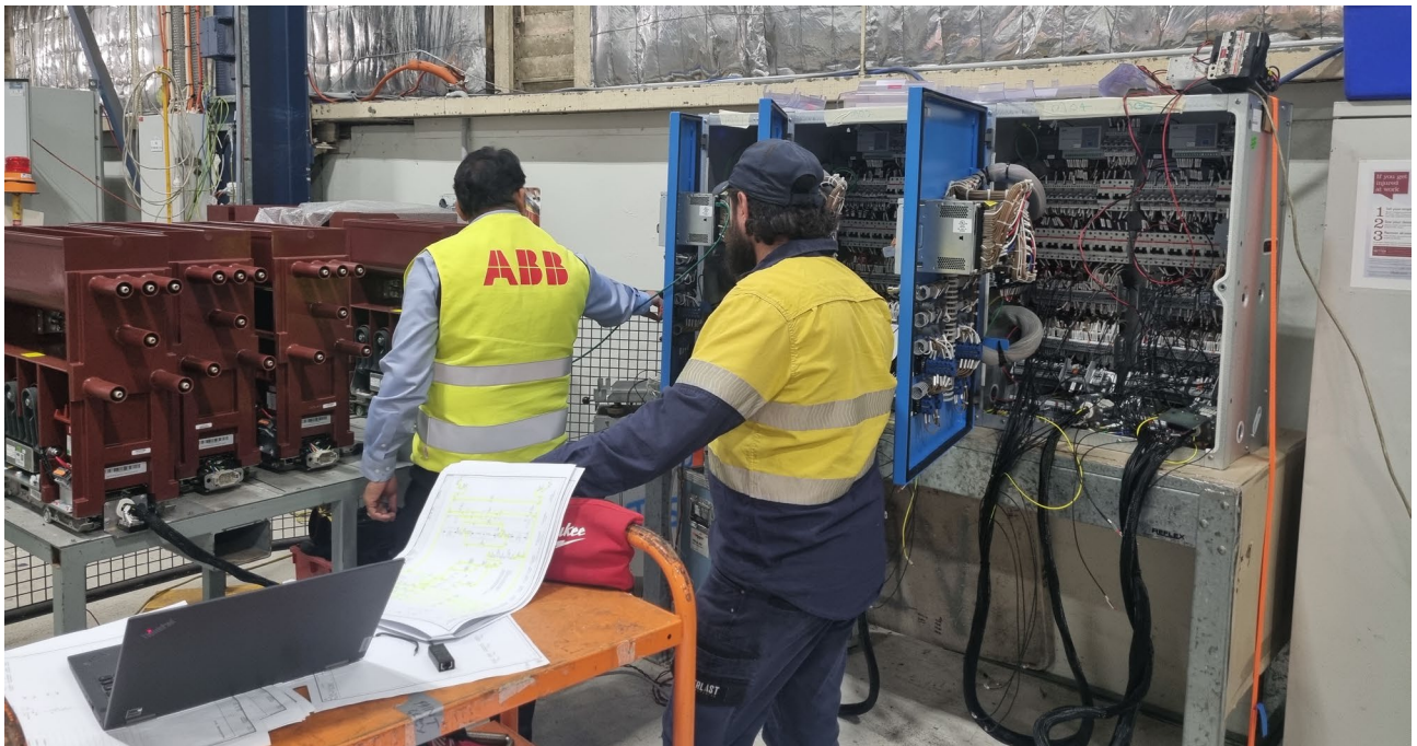
Figure 3 – Factory testing of new remote racking. New motorised contactor "trucks" are at centre left
